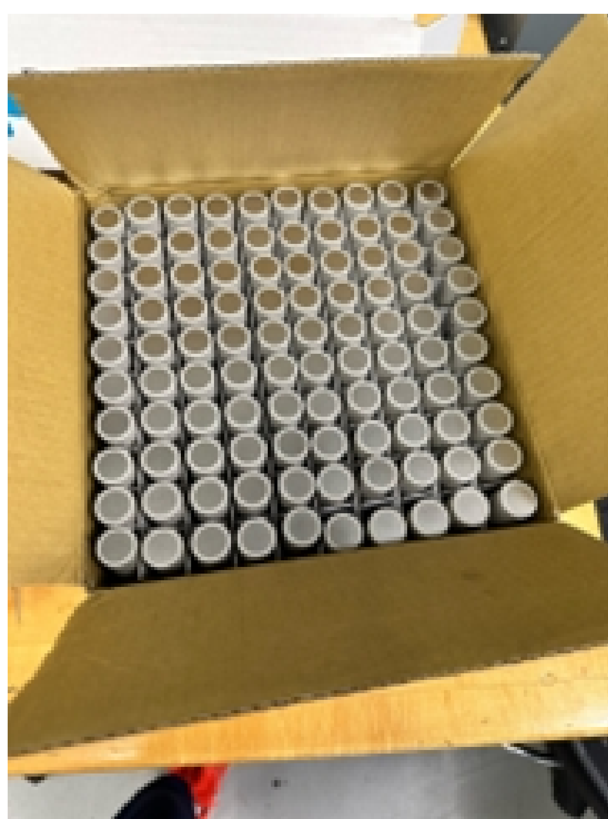
Lithium Ion 2170 cells that go into our module
